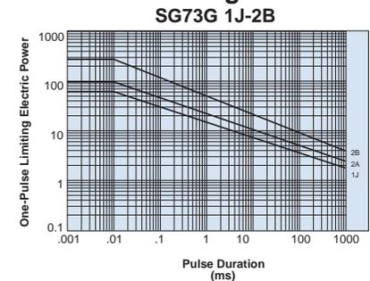
The maximum applicable voltage is equal to the max. overload voltage. Please contact factory for resistance characteristics of continuous applied pulse.
