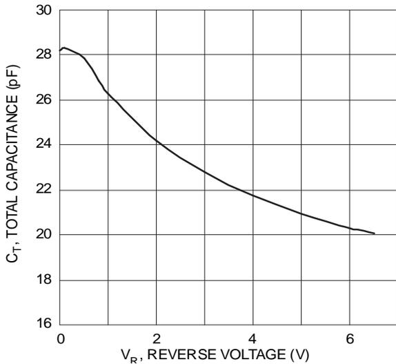
Figure 3. Typical Total Capacitance vs. Reverse Voltage
