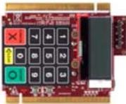
The TWR-POS-K81 development platform is a reference platform for a payment pin entry device. This board includes Cirque SecureSense AFE for secure pin entry. The design files and associated software show an example pin pad application that has been submitted for Payment Card Industry certification. The board is designed to work standalone or as part of the Freescale Tower System.
