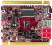
The TWR-K80F150M development board is designed to work in standalone mode or as part of the Freescale Tower System, a modular development board platform that enables rapid prototyping and tool re-use through reconfigurable hardware. Begin constructing your Tower System evaluation board platform today and find additional Tower System boards and compatible peripherals at [freescale.com/Tower](http://freescale.com/Tower).
