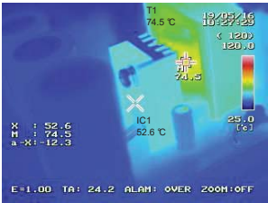
Figure 50-2. Thermal Image "With" Heat sink V IN : 600Vdc, I OUT : 2A
