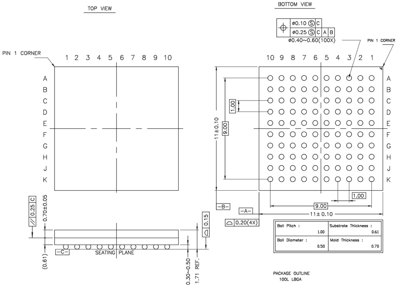
\* THE BALL DIAMETER, BALL PITCH, STAND-OFF & PACKAGE THICKNESS ARE DIFFERENT FROM JEDEC SPEC M0192 (LOW PROFILE BGA FAMILY)
