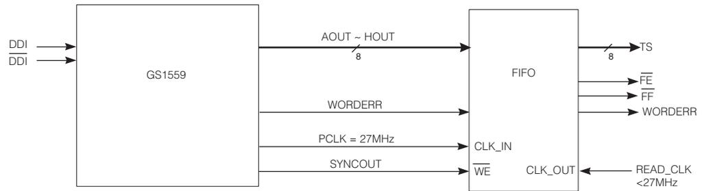
Figure 4-4: DVB-ASI FIFO Implementation Using The GS1559
