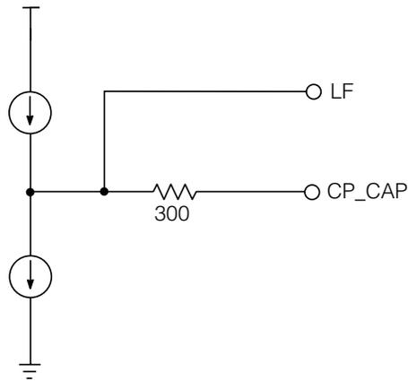
Figure 3-5: VCO Control Output & PLL Lock Time Capacitor
