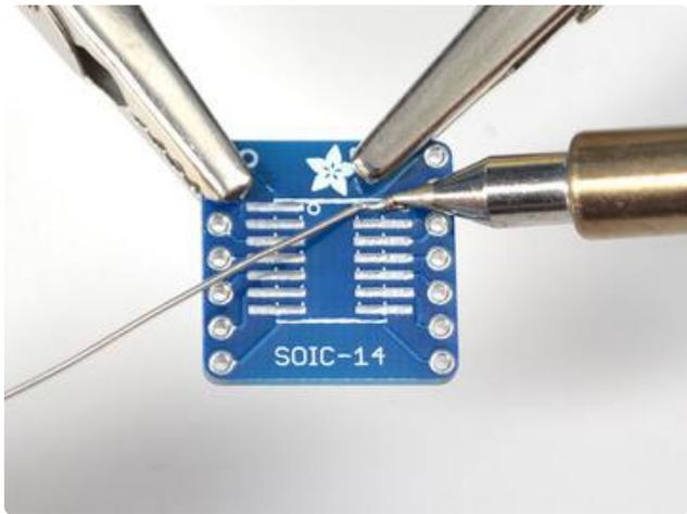
We'll start by melting a little solder on one corner pad. I like going with the top right corner. Melt just a tiny bit on, so its rounded but not blobby
