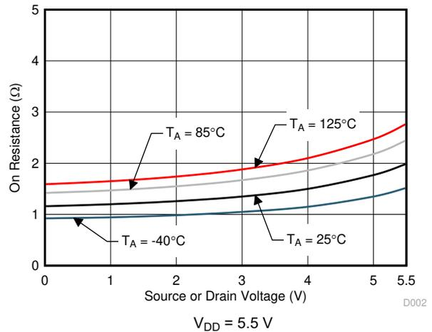
**Figure 6-2. On-Resistance vs Source or Drain Voltage**
