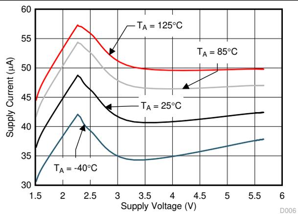
**Figure 6-6. Supply Current vs Supply Voltage**
