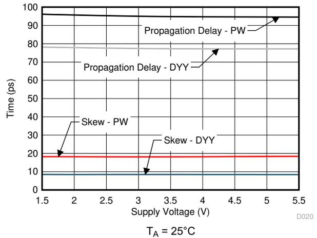
**Figure 6-14. Skew and Propagation Delay vs Supply Voltage**
