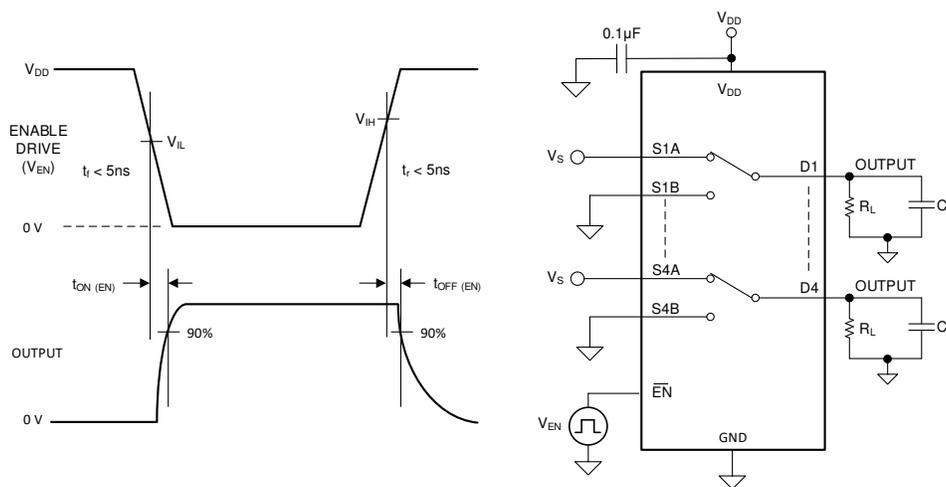
Figure 7-6.  $t_{\text{ON}}(\text{EN})$  and  $t_{\text{OFF}}(\text{EN})$  Time Measurement Setup
