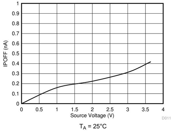
Figure 6-7. IPOFF Leakage vs Source or Drain Voltage
