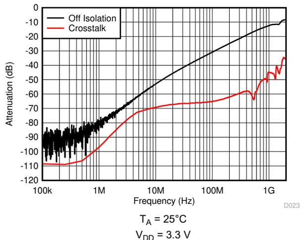
**Figure 6-15. Off Isolation and Crosstalk vs Frequency**
