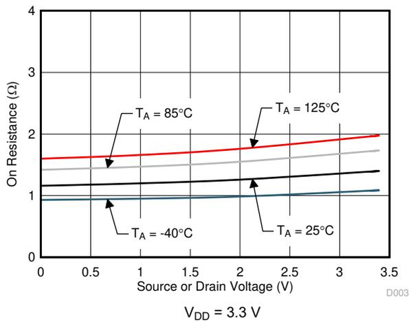
**Figure 6-3. On-Resistance vs Source or Drain Voltage**
