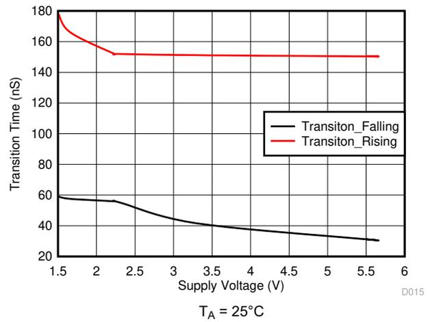
Figure 6-10.  $T_{\text{TRANSITION}}$  vs Supply Voltage
