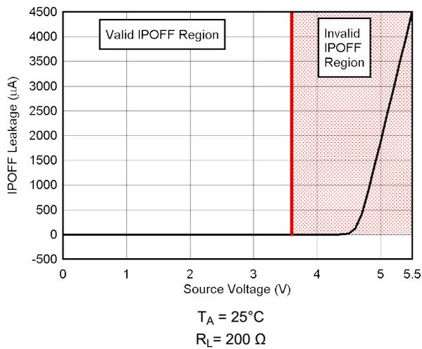
Figure 6-9. IPOFF Leakage vs Source or Drain Voltage
